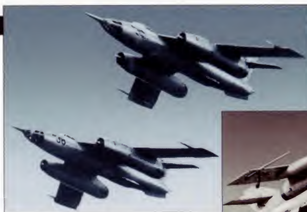
Above: Distinguished by its glazed nose, the 'Brewer' was the first member of the Yak-28 family to enter service. It could carry a hefty bombload and was fitted with a cannon for self-defence and ground strafing. Two fuel tanks (not fitted to these aircraft) could be attached to the outer wings to increase fuel capacity.
